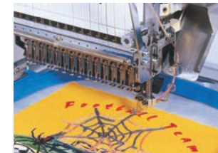
Loop & Cord Device as Cording 当盘带绣装置时, 可转为盘带绣
