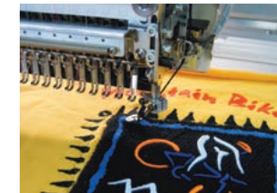
Loop & Cord Device as Looping 当毛巾绣装置时, 可转为毛巾绣
